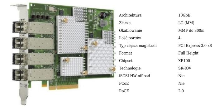
The OCe14000B family of Converged Network Adapters (CNAs) provides high performance 10Gb Ethernet (10GbE) and 40GbE connectivity delivering multiple benefits for the enterprise cloud, including:
