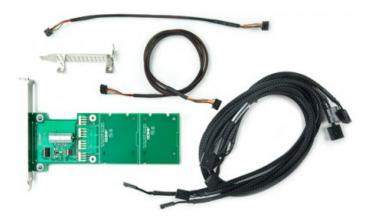
I2C Multiplexer accessory for 9550SXU, 9650SE and 9690SA series RAID controllers.3ware I2C Multiplexer accessory kit supporting SuperMicro backplanes 826TQ, 836TQ, or 846TQ. For use with 9550SXU, 9650SE and 9690SA series RAID controllers.
